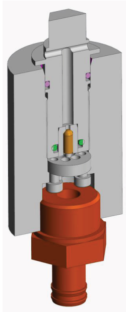
Figure 13: Aeration and Ventilation Unit
