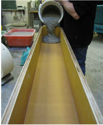
Figure 73: Material testing. LCPC Box: a) equipment, b) final flow shape for the material tested (right). L = 600 mm for SCC3.
