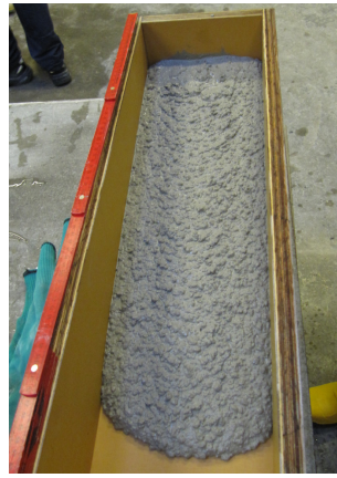
Figure 73: Material testing. LCPC Box: a) equipment, b) final flow shape for the material tested (right). L = 600 mm for SCC3.
