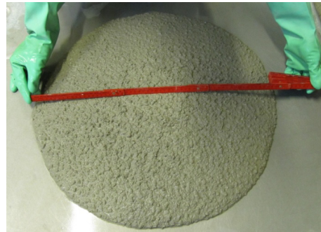
Figure 74: Material testing. Slump flow: a) equipment, b) final shape for the SCC3. D = 570 mm.
