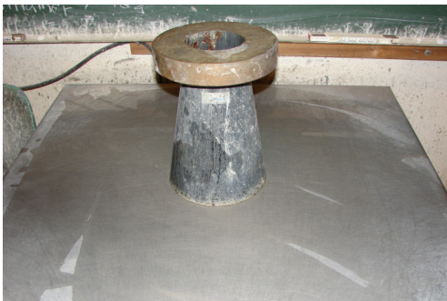
Figure 74: Material testing. Slump flow: a) equipment, b) final shape for the SCC3. D = 570 mm.
