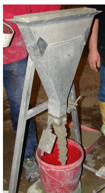
Figure 75: Material testing. a) V-funnel test, b) ConTec Rheometer-4SCC [212].
