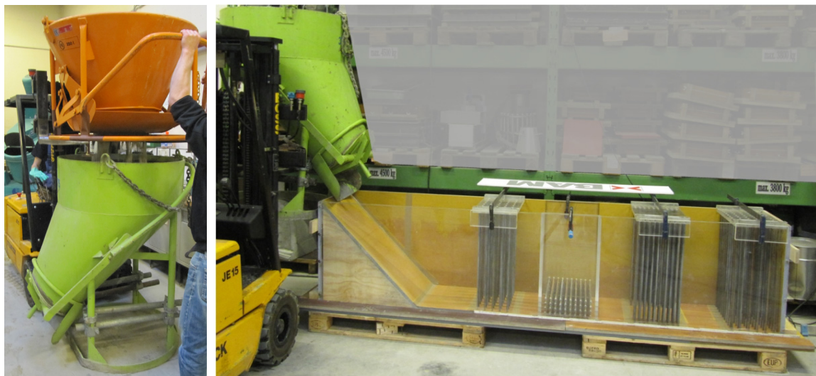
Figure 72: Main experiment: a) filling of the pouring funnel with concrete and transport of concrete to the position above the form; b) the Plexiglas form and the funnel filled with concrete. The experiment starts by pulling a gate on the bottom of the funnel.
