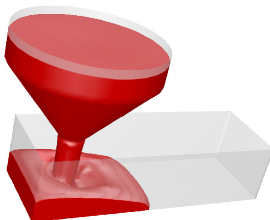
Figure 63: Numerical setup for the calibration of the boundary conditions. Intermediate position of the fluid flowing into the box with no obstacles [14].
