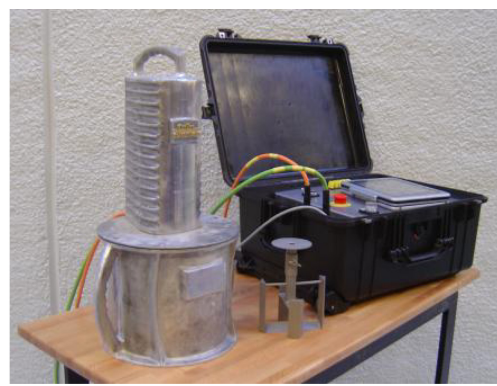
Figure 75: Material testing. a) V-funnel test, b) ConTec Rheometer-4SCC [212].
