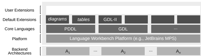
Figure 5. The proposed language ecosystem for cognitive computing based on language workbench technology. The language families are decoupled from the backend architectures and implementation languages.
