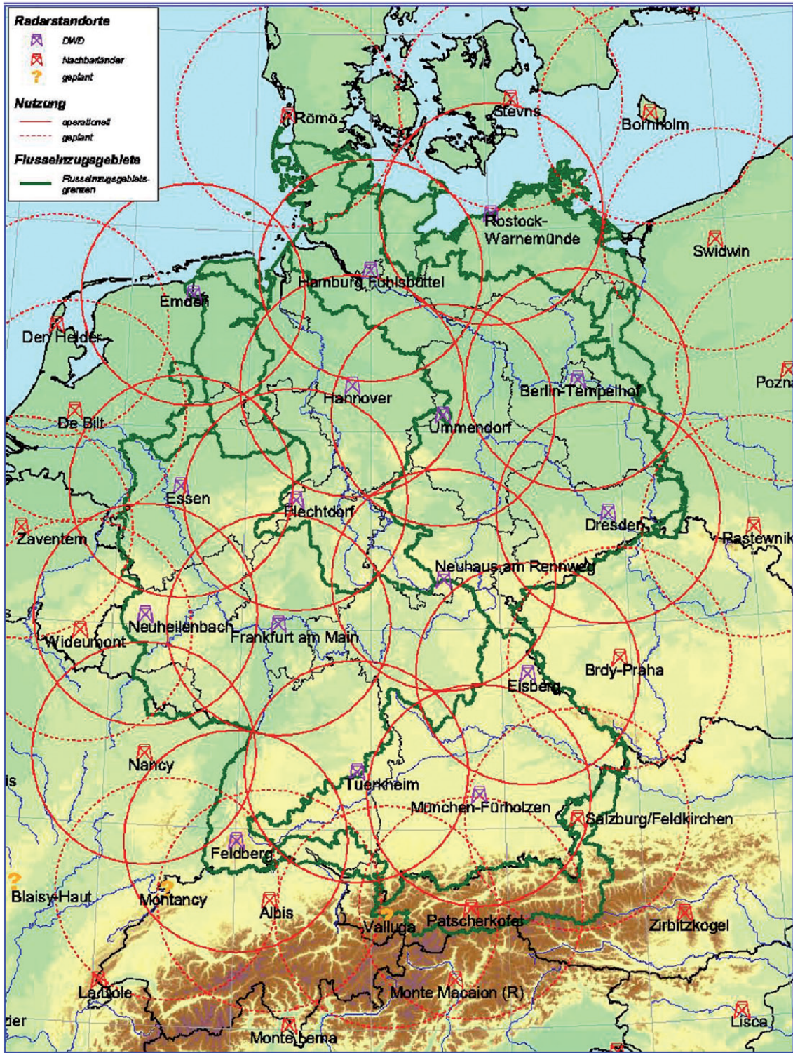
Figure 1.7: Network of C-Band weather radar stations of the German Weather Service (DWD) in Germany and their beam coverages. The figure was taken from Weigl and Winterrath (2009).
