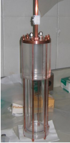
Figure 6.42: Acrylic vessel, or bucket source , with a hollow space of \sim 11 for liquid scintillator. The vessel was built for deployment in the water-filled SNO(+) detector to test optical properties of LAB scintillator. The picture is taken from [248].
