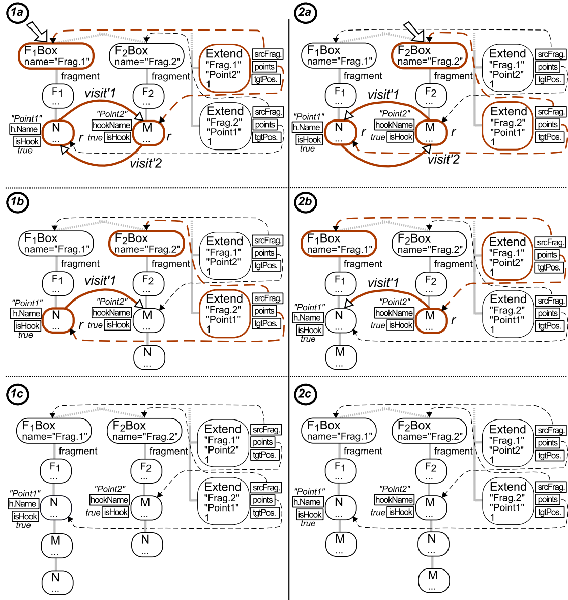
Figure 5.11.: Attribute-determined composition can yield different results depending on where the ReRAG evaluation starts.
