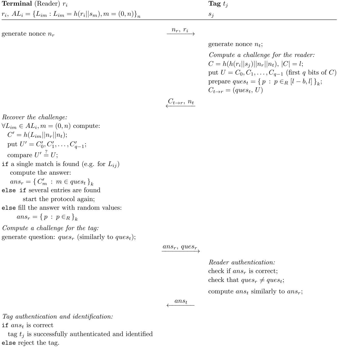
Figure 4.8: TanSL-1. C_x denotes the x -th bit of a bit string C .
