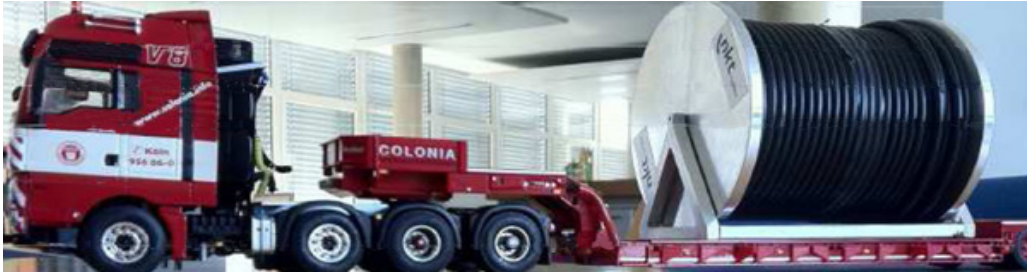
Figure 55: Flat-bed trailer concept with longer cable drum length wise. Picture: nkt cables.
