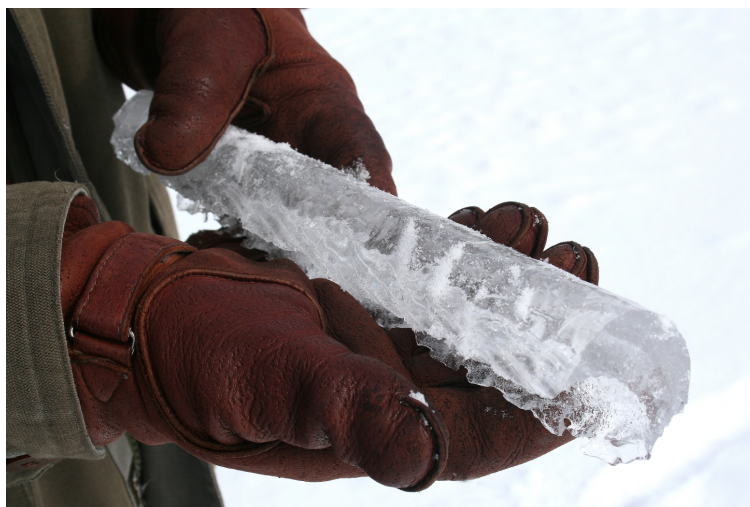
Figure 36: Piece of fallen ice from a transmission line.
