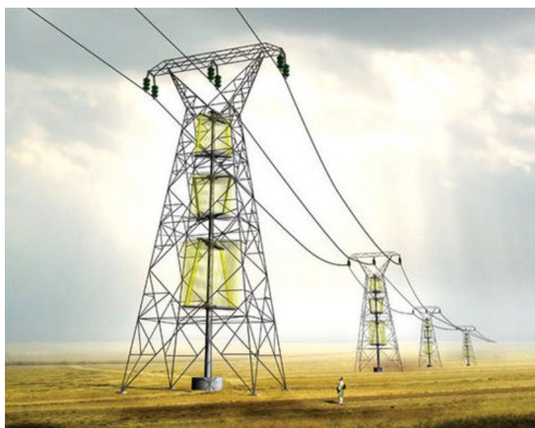
Figure 61: Transmission pylon with integrated small-scale wind turbines. Picture: Wind-In.
