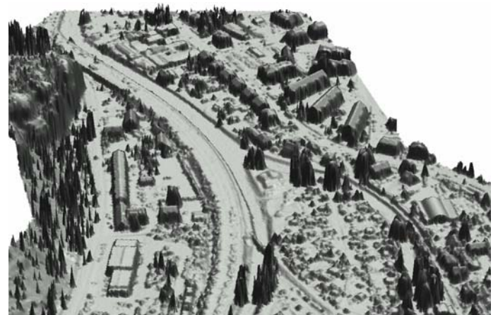
Figure 2. Morphological data set with vegetation and buildings from laser scan (confluence of the rivers Wilde Weißeritz and Rote Weißeritz at the town of Freital; data: LTV 2005).
