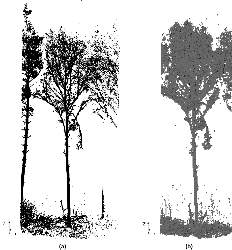
Figure 5.5: A tree from data set B as (a) 3D point set and (b) corresponding voxel representation.
