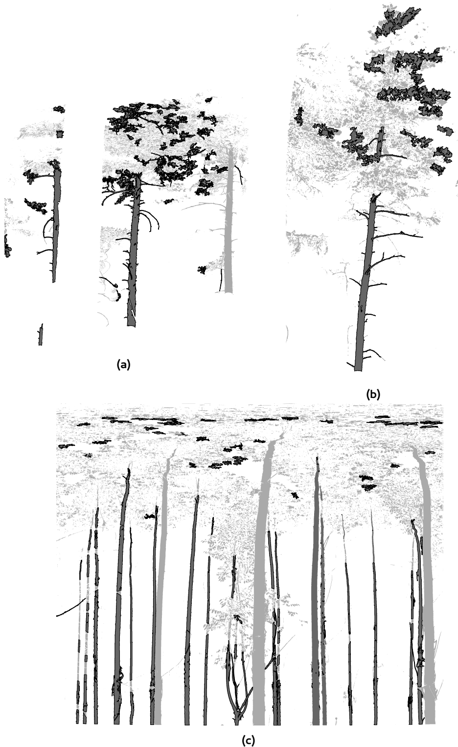
Figure 6.13: Results of the experiments on data set P in subfigure (a) and (b), and on data set E (c). Components that have been processed are drawn in dark gray. Retrieved boundaries are drawn as black lines. Components in light gray have been omitted in the experiments. A case when the main boundary has not been found is visible in the right section of subfigure (c).
