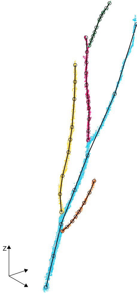
Figure 7.9: The segmentation from figure 7.6d is colormapped to the 3D point set. The 3D polylines that are the result of the PLA on the point groups are shown in black.
