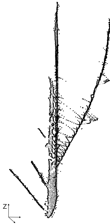
Figure 6.14: The Faro Focus 3D samples points between branch and trunk surface that are apparently floating in the air and do not represent actual surface samples. These spurious points hinder tracing of the rift between branch and trunk to the full extend.
