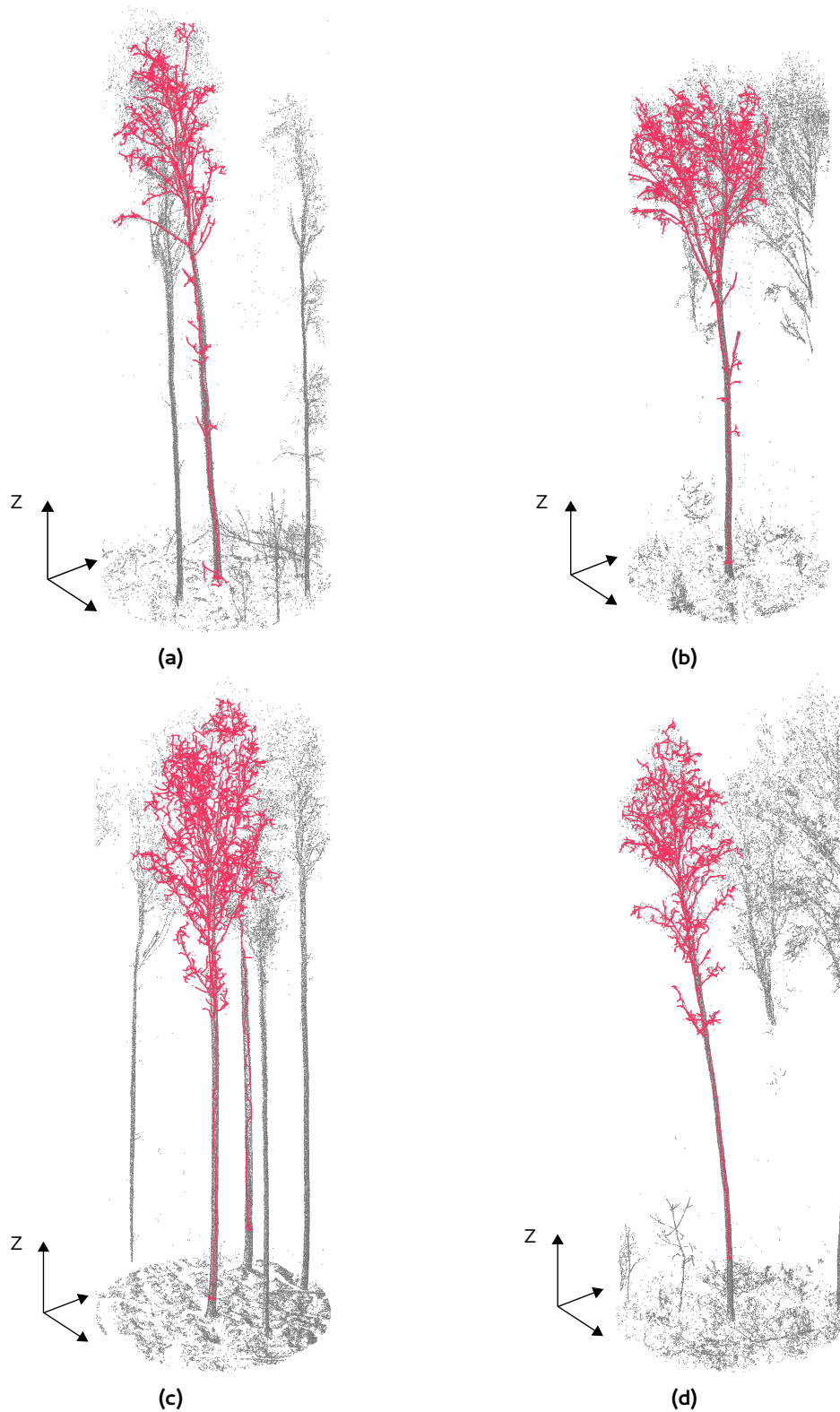
Figure 5.8: Results of the experiments. The retrieved skeleton graph is drawn in red as overlay onto the 3D point set in gray. Subfigure (c) shows a case where the neighboring tree trunk is included in the skeleton due to intertwined crowns.
