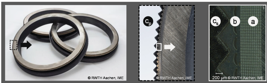
Figure 8: Sliding sealing ring with microstructured functional surfaces
