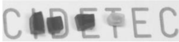
Fig. 5.7 - From left to right sequence of photographs for the obtained thermosets with poly(0), poly(1), poly(2) and poly(3).
