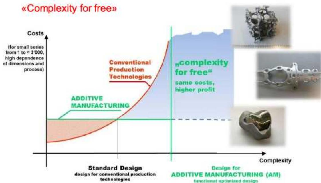
Fig. 2.1.2. Advantages of the additive manufacturing technologies [Ema13a].
