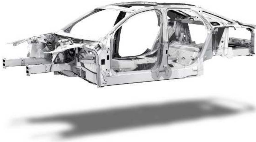
Fig. 1.1.1. Structure of a car, where the skeleton is made of Al-based alloys [NYT12a].
