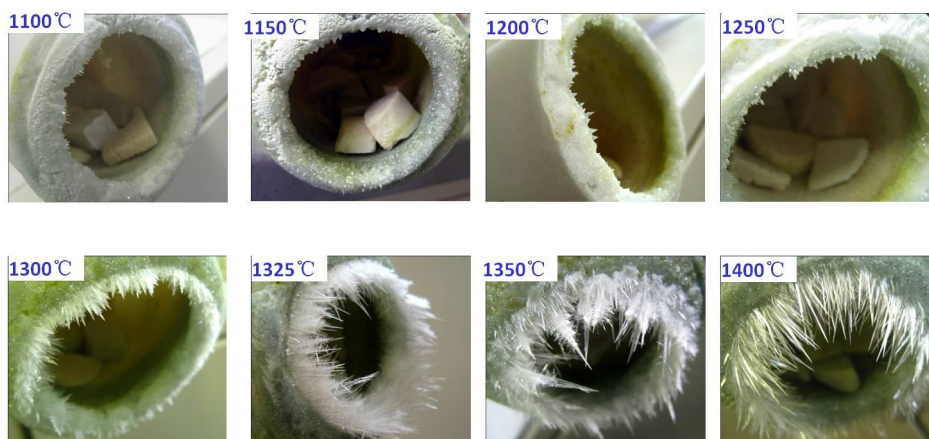
Figure 4.13: The growth of ZnO crystals by vapor phase method at different temperatures while keeping other parameters the same.
