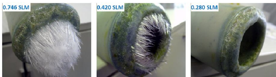
Figure 4.14: The growth of ZnO crystals by vapor phase method at different N_2 flow rates while keeping other parameters the same.
