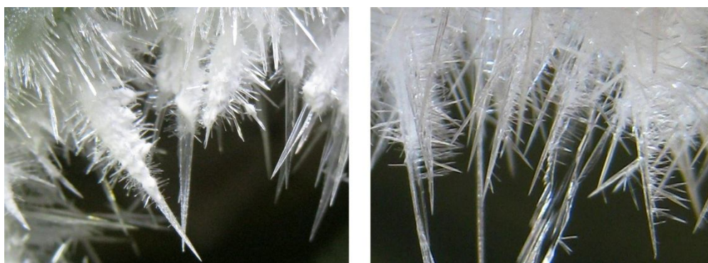
Figure 4.20: Dendritic growth by high supersaturation of zinc vapor
