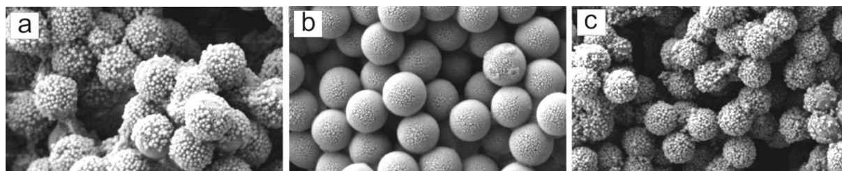
Figure 31. Scanning electron microscopy images of layers formed on silicon wafers after evaporation of the solvent from a particle dispersion: (a) raspberry-like particles with initiator (RP100-BrIn); (b) spherical particles with grafted PPFS (SP1000-PPFS), and (c) raspberry-like particles with PPFS (RP100-PPFS)
