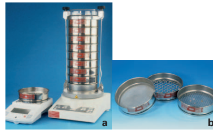
Fig. 2. Sieve tower with scales (a), individual sieves with different mesh widths (b).
