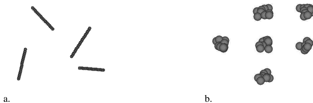
Figure 5.14: Schematic view of already developed and implemented into PFC a) fibres and b) coarse aggregates
