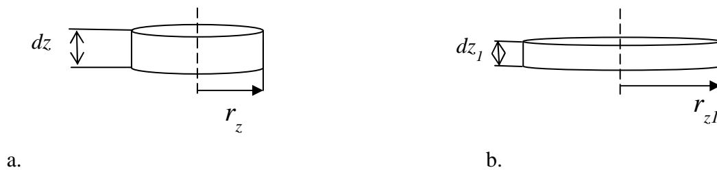
Figure 3.8: Change in layer of thickness dz : a) before and b) after lifting the cone
