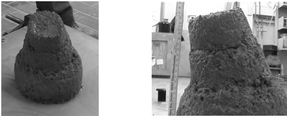
Figure 3.9: The slump test of an ordinary concrete mixture. In this experiment the part of slump cone without deformation is observed; the undeformed part of the concrete has some inclination
