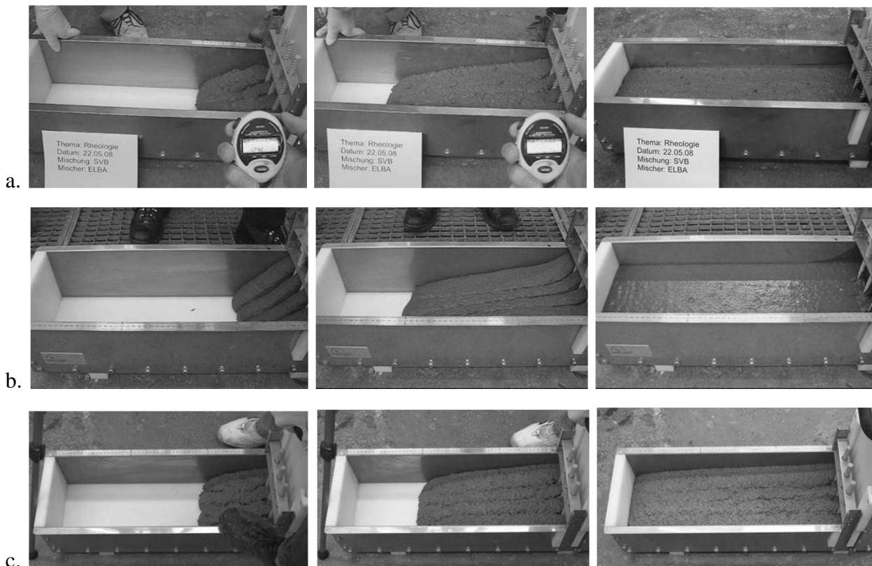
Figure 3.5: Images from L-box tests with a) SCC, b) UHPC1 and c) SCLC
