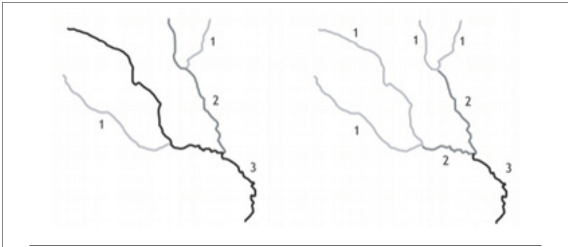
FIGURE 2.11: Comparison between Horton (left) and Strahler (right) principles of ordering streams. Figure taken from (Cecconi 2003).
