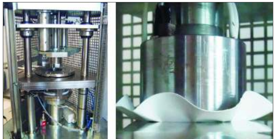
Fig. 6: Test equipment for deep drawing of paperboard at TU Dresden
