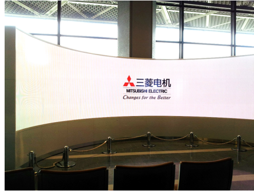
Figure 1.1: Photograph of the world's first 160° OLED panorama display (9.6 x1.9 m) at Tokyo airport fabricated by Mitsubishi Electric and installed in June 2012.
