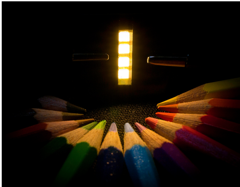
Figure 9.13: Photograph of four operating white tandem OLEDs on NW electrodes. The picture has been taken by Caroline Murawski.
