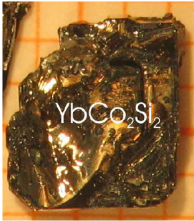
Figure 4.48 – Photography of a \text{YbCo}_2\text{Si}_2 single crystal on millimeter paper.
