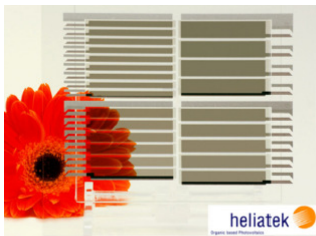
Figure 3.10. A photograph of the semi-transparent OPV cell with an efficiency of 4.9 % and transparency of 24 %; taken from [132].
