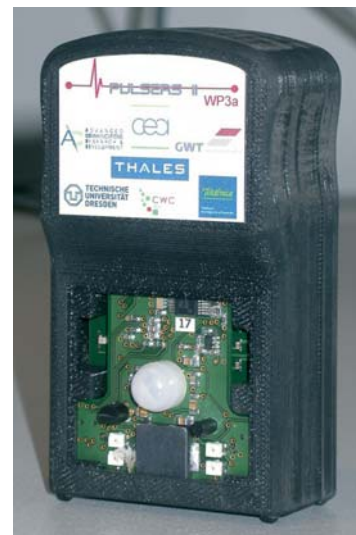
Fig. 4: Prototype of a UWB-sensor Photo: Benoît Denis, CEA-Léti, France
