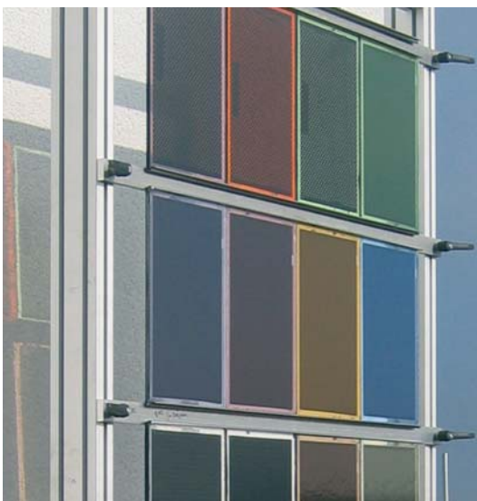
Small samples of semi-transparent and opaque CIS thin film solar modules produced in coloured and patterned laminated glass. (Photo: ZSW)
