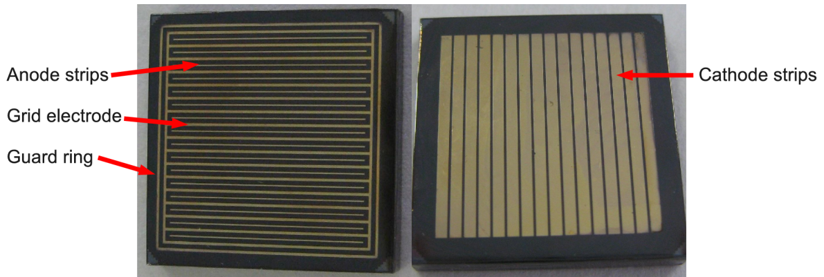
Figure 3.3: Left: anode electrode of the CdZnTe detector. Right: cathode side (images by Baltic Scientific Instruments).
