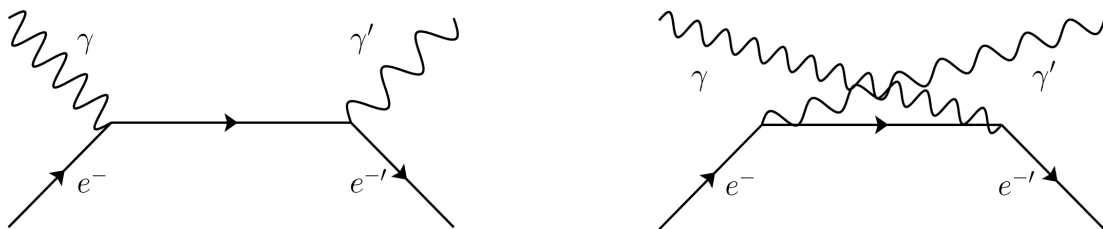
Figure 1.1: The two Feynman graphs of Compton scattering (first order, s - and u -channel).
