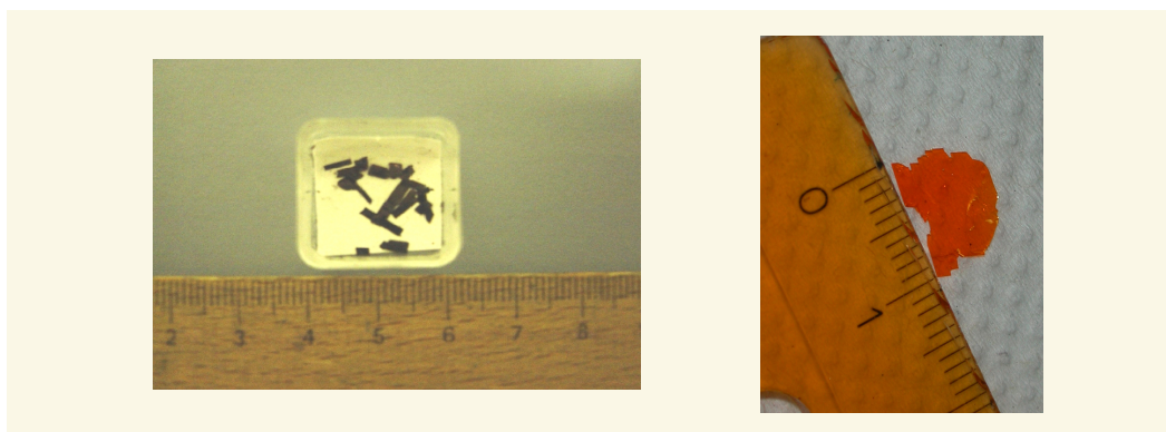
Figure 2.8. | The pentacene (left) as well as tetracene (right) crystals as obtained by sublimation from the gas phase.
