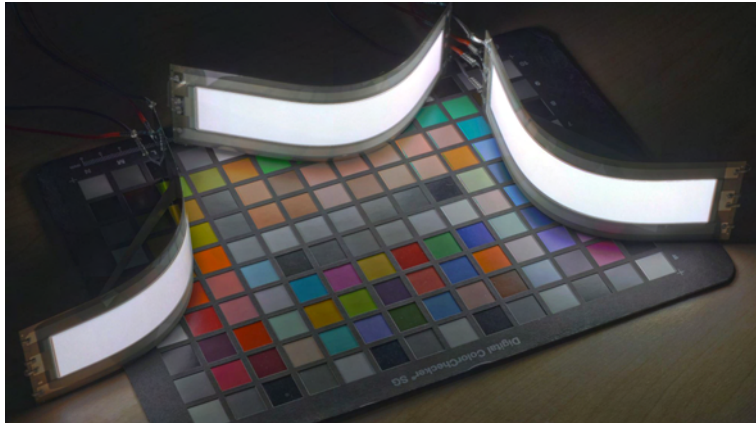
Figure 1.1: High quality white light emitting OLED on metal substrates demonstrated by OSRAM in November 2011. The luminous efficiency is 32 \text{ lm/W} at a brightness of 1000 \text{ cd/m}^2 . Image taken from [5].
