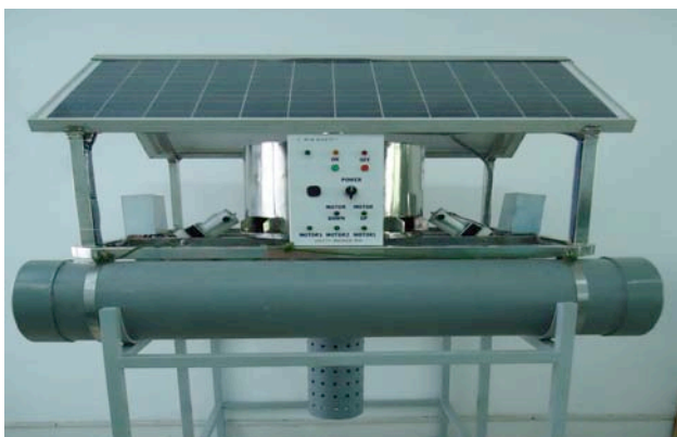
Figure 7. Autonomous water cleaning machine using solar energy
