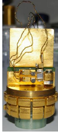
Figure 3.3: Experimental cell for electrical resistivity, thermal conductivity and thermopower measurements at low temperatures.
