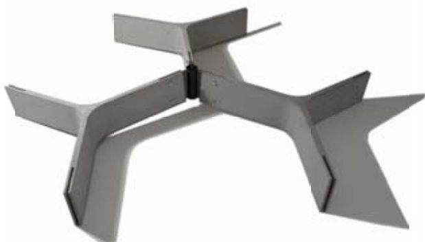
(a) Bauteil­fü­gung der Y-Elemente (a) Joining of Y-shaped elements
