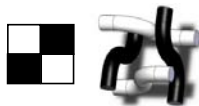
Figure 18: Weave representation of a plain woven fabric (left) and actual positioning of warp (black color) and weft (white color) yarns (right)
