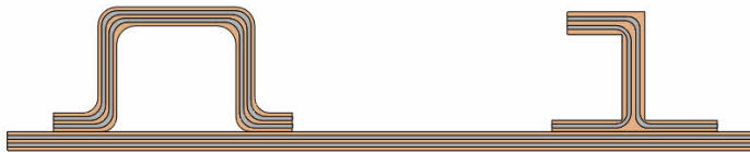
Figure 16: Stiffener structures for aerospace applications (above) and schematic of stacked fabric layers (below) where different color means separate layers [32]
