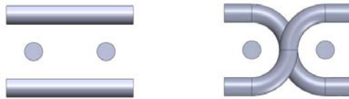
Figure 23: Side-view of patterns with two warp yarns and two weft yarns. Floating of warp yarns without forming a woven structure (left), plain woven structure (right)
