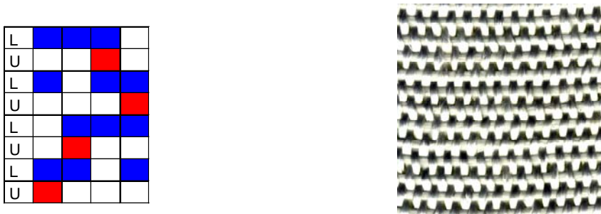
Figure 41: X-twill weave (left) L: lower weft yarn, U: upper weft yarn, and woven fabric (right)
