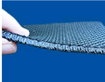
Figure 8: Warp knitted spacer fabric [14]
