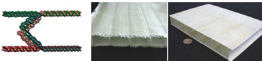
Figure 75: U-shaped spacer fabric from concept to sandwich composite; CAD (left), woven preform (middle), composite (right)
