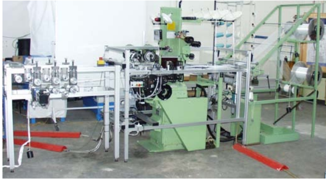
Figure 13: Modified narrow weaving machine [21]
