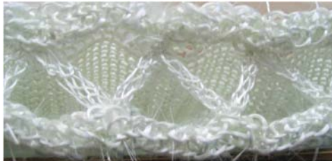
Figure 12: Weft knitted spacer fabrics with knitted cross-links [20, 21]
