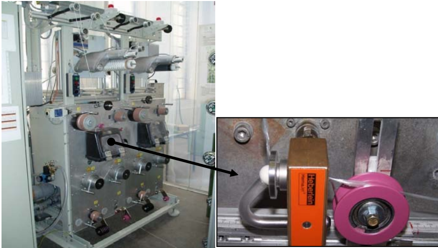
Figure 29: Air-jet texturizing machine utilized for commingled yarn production (left) and detail view of the air nozzle (right)
