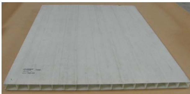
Figure 76: Sandwich composite component from spacer fabrics
