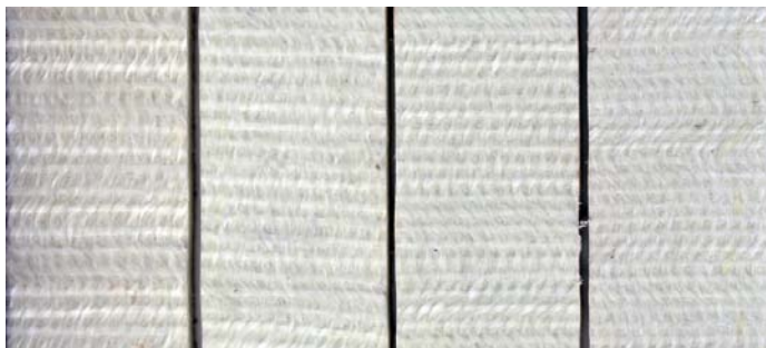
Figure 45: Composite surfaces with weft densities of 7 to 10 from left to right
