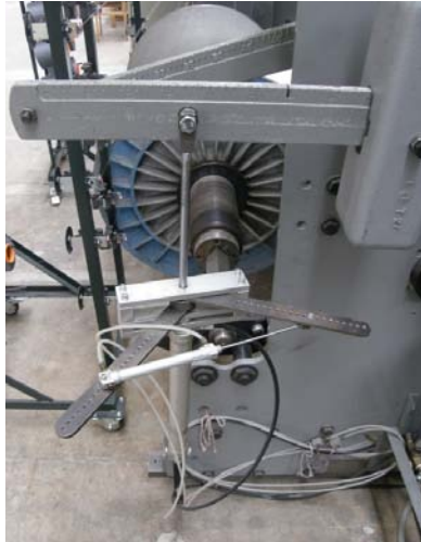
Figure 69: Warp yarn pull-back mechanism
