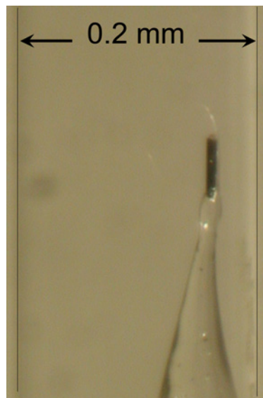
Figure 6.14: A single crystal of \text{La}_{3.67}[\text{Ru}(\text{C}_2)_3] mounted on a glass capillary.
