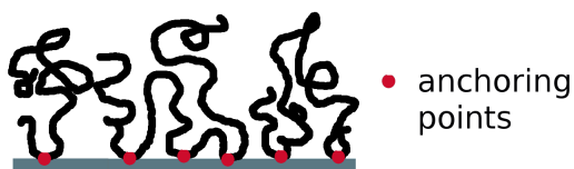
Figure 2.3.: Scheme of a Guiselin brush where the polymer chains are immobilized via more than one anchoring point along the chain.
