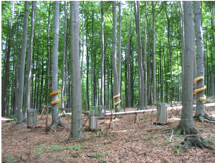
Figure 2.2 Measurements of canopy drip and stem flow at the Beech site (visible: throughfall troughs with storage tank as well as spiralled collectors and storage tanks of stem flow measurements)
