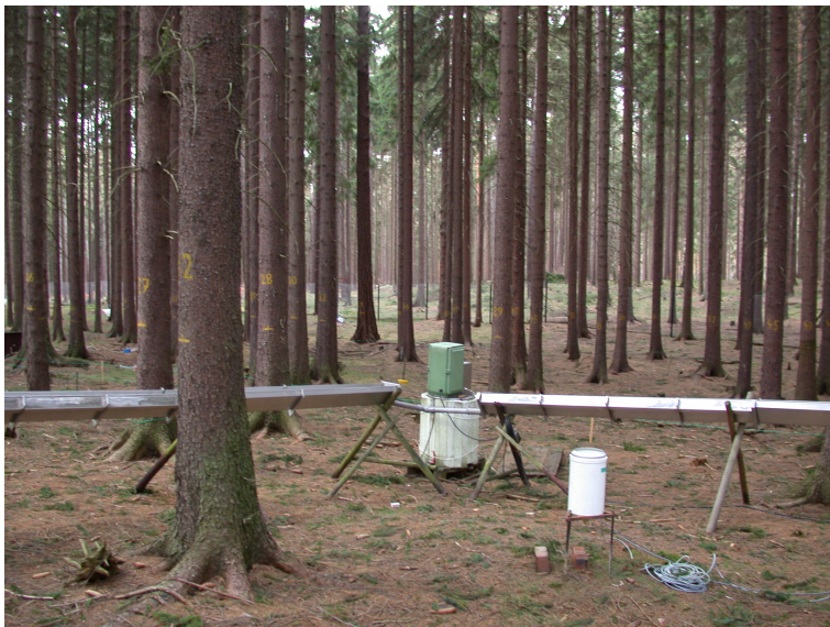
Figure 2.3 Measurements of canopy drip at the Spruce site (visible: throughfall troughs with storage tank and one of additional bucked rain gauges for estimation of spatial distribution of canopy drip)
