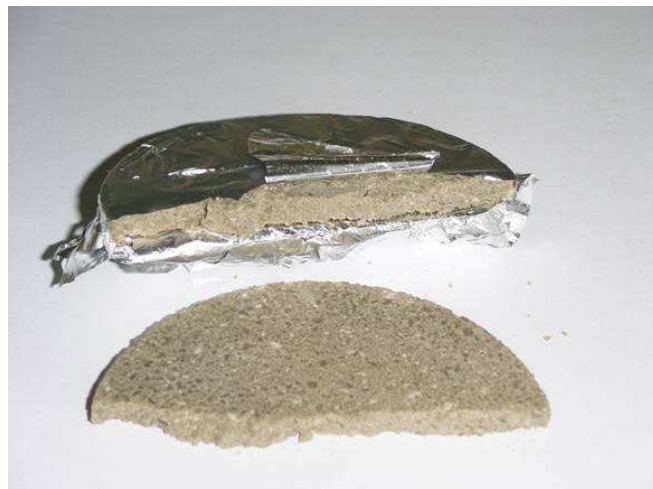
Fig. 3.12. Photo of an opened paraffin pellet which was wrapped and glued into aluminium foil.
