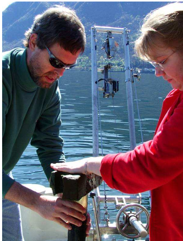
Fig. 3.7. Closing the PVC-tube with the sampled sediment material using a soft foam material with absorbing properties.
