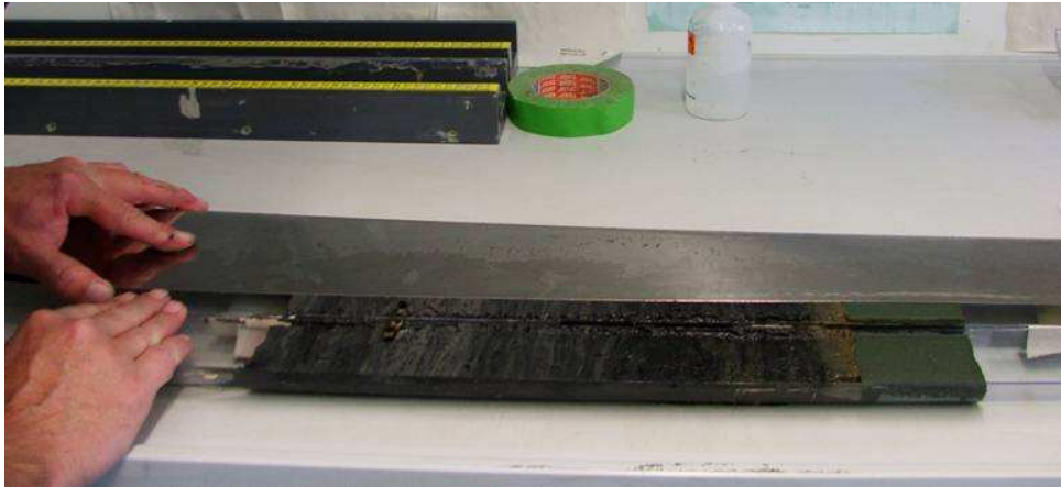
Fig. 3.8. Preparation of the sediment samples: lengthwise cut of the sediment core using metal sheets.
