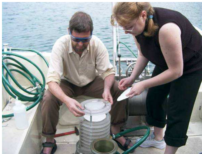
Fig. 3.4. Installation of filter sets for large volume water sampling using the “Midiya” system.
