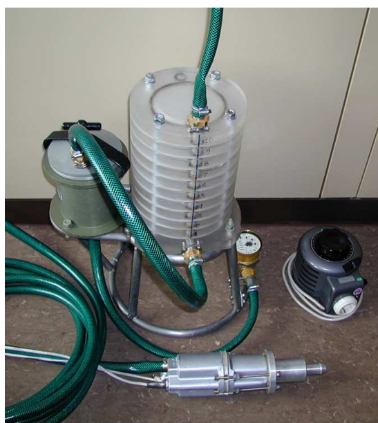
Fig. 3.3. Large volume water sampler “Midiya” with a pump (in front), a block for filters (in the middle), a chamber for adsorber (left); and a transformer (right).
