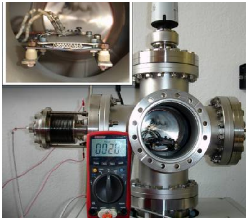
Figure 3.4: UHV annealing chamber at FZD with a view on the sample holder (inset).
