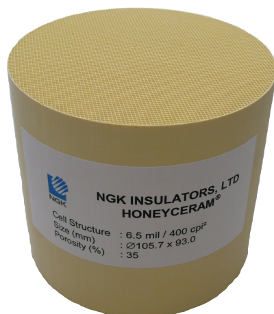
Figure 4.1.: Cordierite monolith, supplied by the company NGK .
