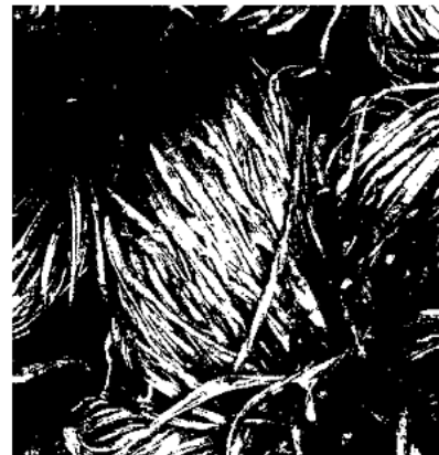
Figure 3.1 Sensibility comparison between CWL and SDCM sensors by the same sample, which corresponds to a cotton fabric surface (sampling interval = 626 \mu\text{m} ). White regions represent valid (measured) points, while black regions represents invalid (no detected) points.
