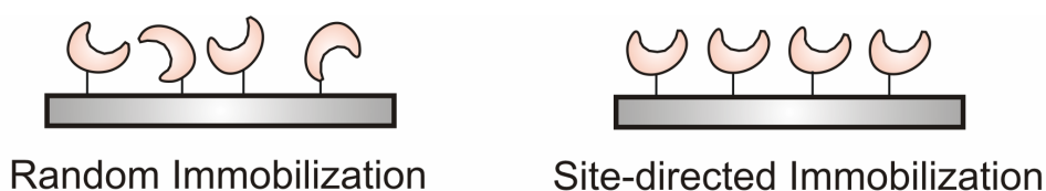
Fig. 3.11. Schematic representation of random and site-directed enzyme immobilization. The active site of the protein is shown as an indentation. In random immobilization, the active site may be partially or totally blocked whilst in site-directed immobilization all active sites are fully accessible to the substrate (adapted from Wang et al. 2001 [155]).
