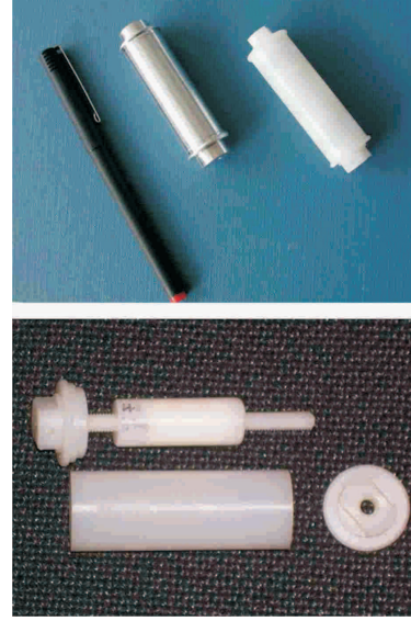
Figure 4.17: The cassettes used for mounting targets in measurements with rabbit system. a) The cassettes (either made of polyethylene or aluminum), compared to a pen to have a feeling of the dimensions. b) The cassette with Sm target mounted. The target is \text{Sm}_2\text{O}_3 powder filled into a cylinder with dimensions given in Table. 4.1.
