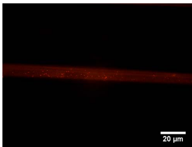
Figure 4.13: Self-rolled P4VP/PS tube with PSA molecules labeled by Rhodamine 6G dye
