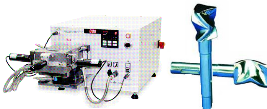
Figure 3.1 Brabender plasticorder: (left) the mixing chamber and (right) sigma type screw used for melt-compounding
