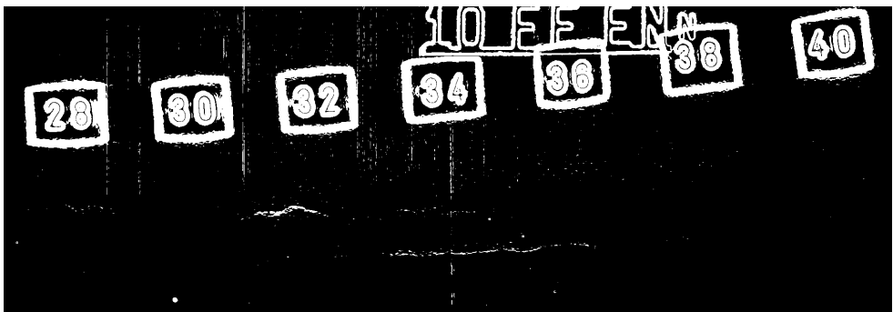
Figure 2.3: Result of application of Nevatia-Babu operator to the image from Fig. 2.1 and subsequent thresholding operation with manually selected threshold.
