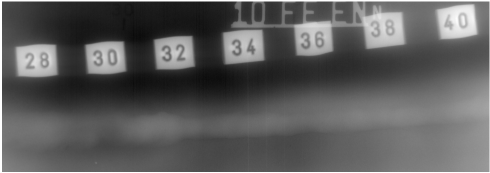
Figure 2.1: Part of typical radiographic image of welding seam. Lead markers (numbers in white squares) show the circumferential weld position in cm. A crack indication is located at position 32-39 under the seam.
