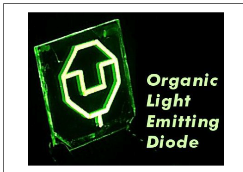
Figure 1: An organic LED showing the logo of the Technical University of Dresden.
