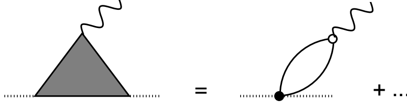
Figure 4.6: Effective spin-phonon coupling vertex. The dominant contribution shown on the right stems from a combination of spin-orbital (filled dot \propto t ) and orbital-lattice (open dot \propto g_2 ) coupling vertices. The orbital susceptibility depicted by a bubble controls the coupling strength. Solid, dotted and wiggled lines represent orbiton, magnon, and phonon propagators, respectively.
