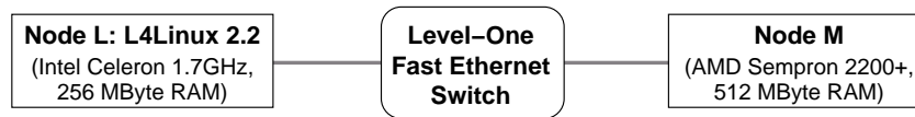
Figure 45: Setup for Section 7.4.7: two nodes ( L , M ) are connected to a Fast Ethernet switch. Node L executed L 4 Linux: Once the standard L 4 Linux with its native network stack and NIC driver, another one it executed L 4 Linux with the RT-Net driver stub. Node M generated test traffic to and received test traffic from L . For the RT-Net setup, it executed the bandwidth manager.
