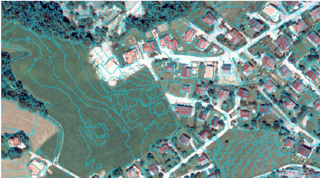
Figure 2-1: Segmentation result (blue polygons) of LiDAR data using eCognition with underlaid aerial imagery and map information (red polygons)
