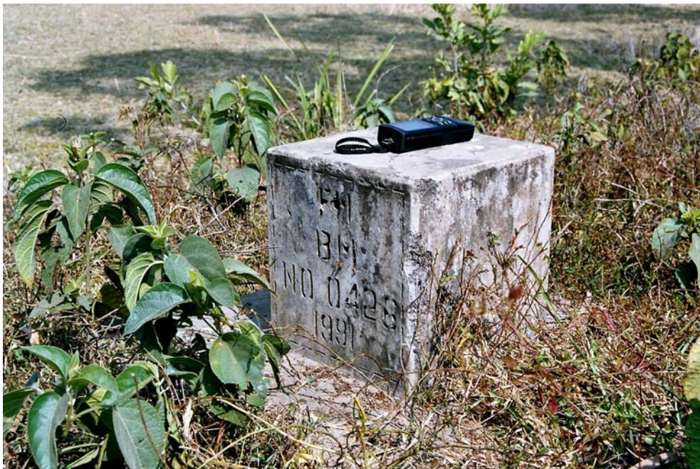
Figure A-II. Geodetic pillar and acquiring geographic position by a handheld GPS
