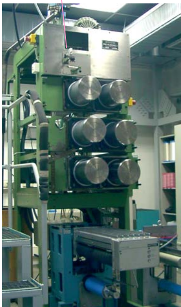
Figure 2.1.1 (a) Piston equipment (b) extruder equipment for melt spinning in IPF Dresden
