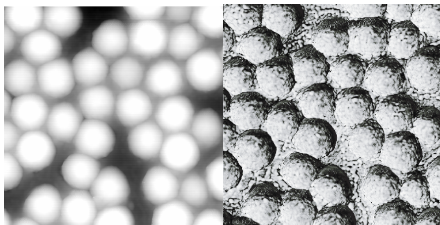
Figure 5.7. AFM topographical (left) and phase (right) ( 1 \times 1 \mu\text{m}^2 ) images of the silica nanoparticles with grafted block copolymer brushes on the surface of silica wafers.
