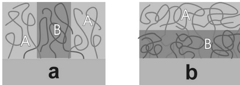
Figure 2.2. Schematic representation of phase segregation of a mixed polymer brush.
