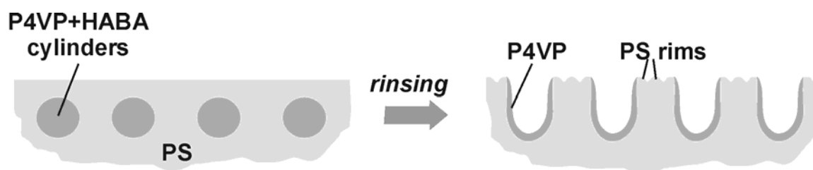
Figure 4.10. Sketch showing the transformation of the parallel P4VP+HABA cylinders into the grooves.
